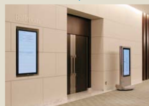
The two displays on the banquet floor list the scheduled events of the day to allow at-a-glance recognition of destination rooms (at left in photo). Movable stand-integrated display units are also utilized (at right in photo).
