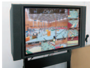
▲ Displayed images can be split into several windows to allow an athlete's motion to be viewed from various angles.
